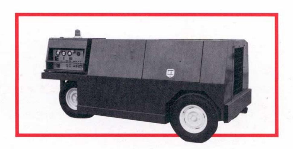
Stewart & Stevenson electrical ground power units are available in either trailer, truck or tow-tractor mounted models, ranging from 37½ KVA to 200 KVA. Also available are Air Start units ranging from 120 PPM to 400 PPM and Tow Tractors in both Diesel and electric driven configurations, ranging from 16,000 to 100,000 lbs. GVW. Stewart & Stevenson backs it's equipment with complete Parts and Service Responsibility around the clock, anywhere in the world.
